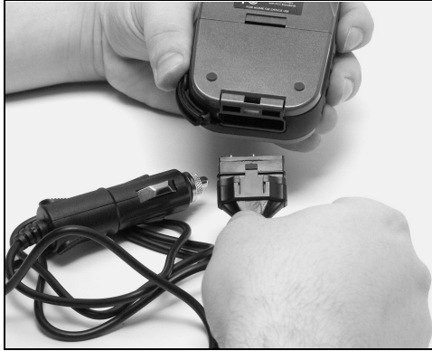
Attach external power cable to the iFINDER.
